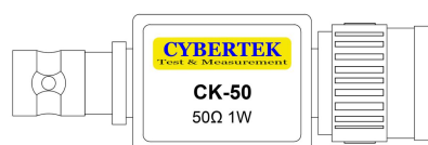
Figure 4 BNC-male-to 50 \Omega load
